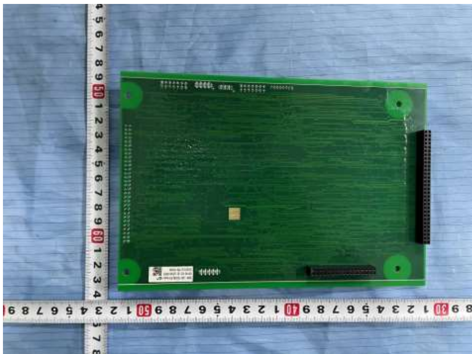
Solder side of control board for all models
