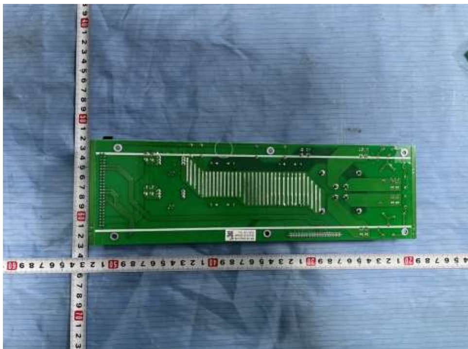
Solder side of PV board for all models
