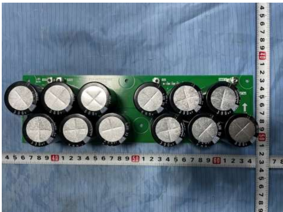
Component side of capacitance board for all models
