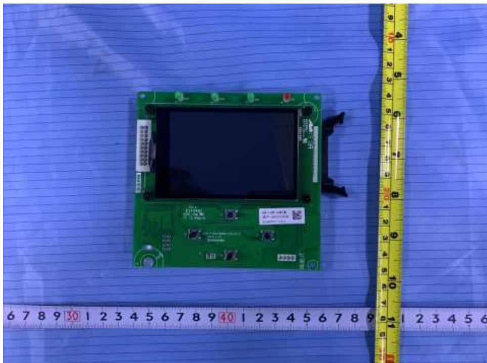
Component side of LCD board for all models
