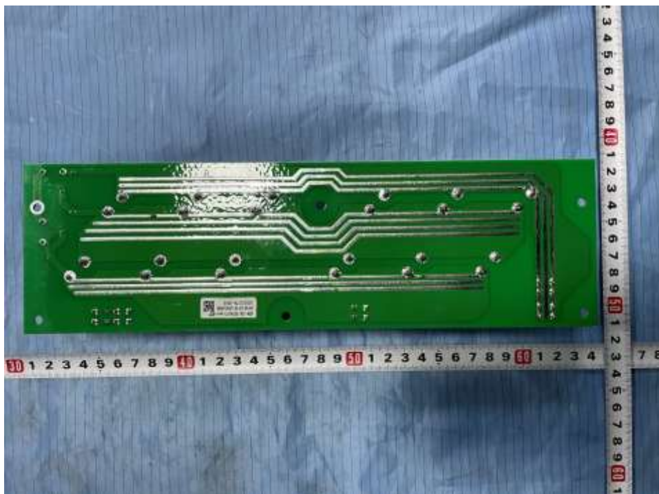
Solder side of capacitance board for all models
