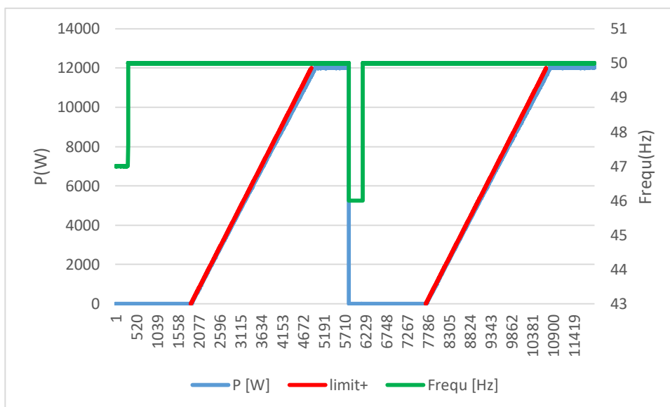
Graph of the gradual power supply : Test e) for \geq 47,50\text{Hz}
